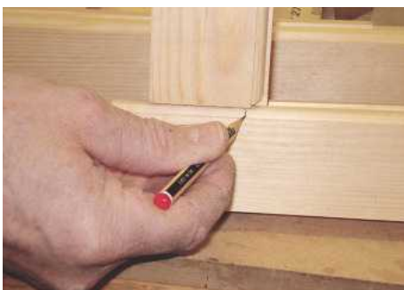
▲ Pic.19 The rails are offered up to the stiles, which are marked...
